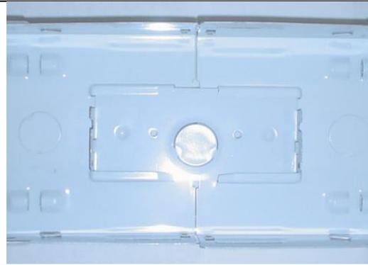
5. **8' TANDEM STRIPS ONLY.** Insert the lamp holders into the center socket plates. The socket plates insert into the center slots just as they do on the fixture ends. The lampholders will be back-to-back. The two Red leads should go into the same socket plate. The two Blue leads should go into the other socket plate. When all socket bars and end caps are installed snap the front cover(s) onto the fixture.
